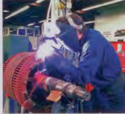
Rotor Bar Welding & Rebaring
