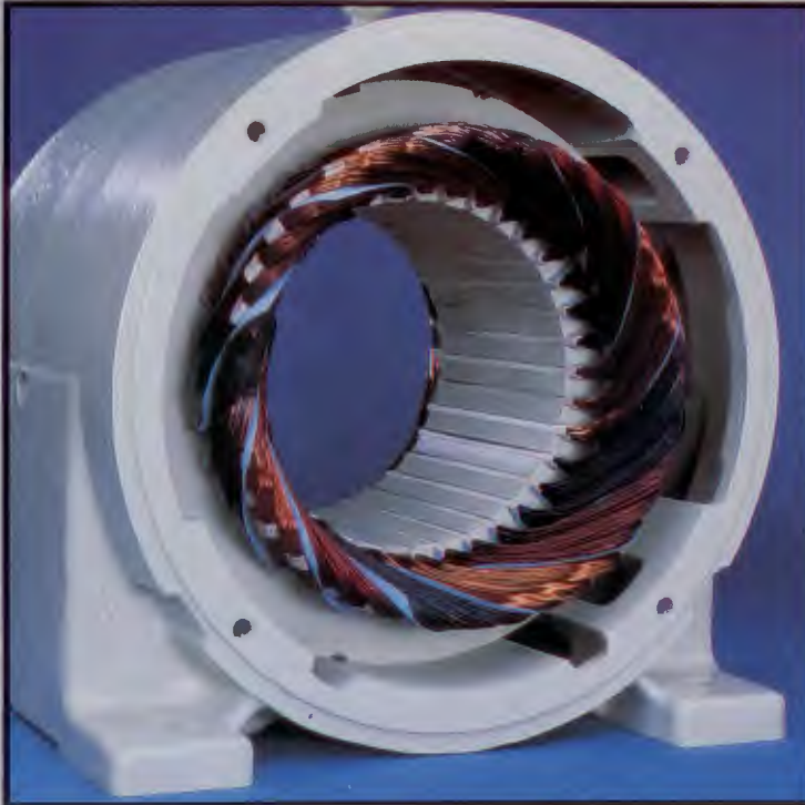
9 Phase Damage Due to Unbalanced Voltage
