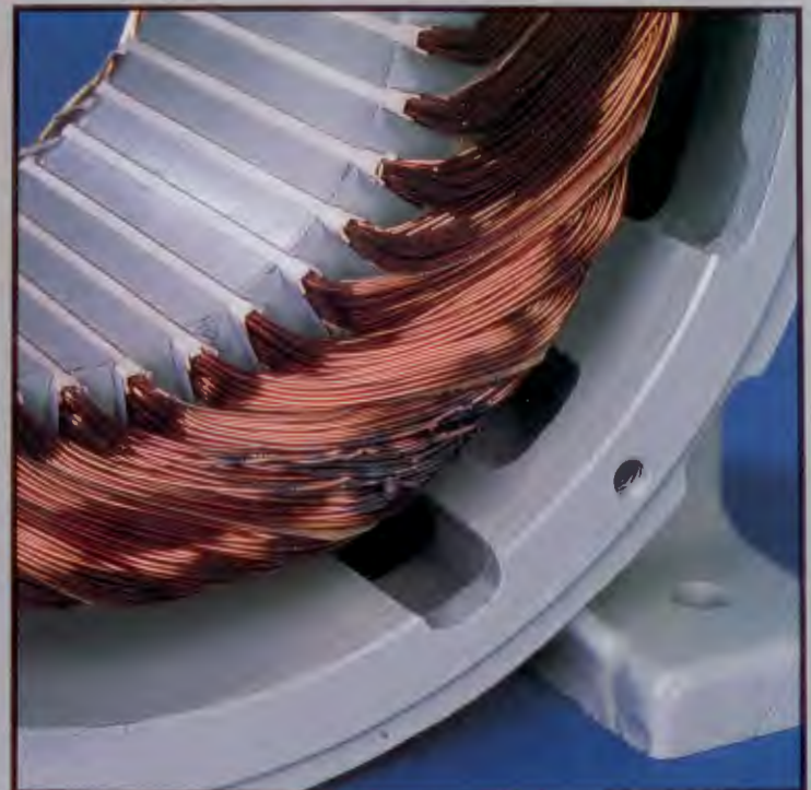
4 Winding Shorted Turn-To-Turn
