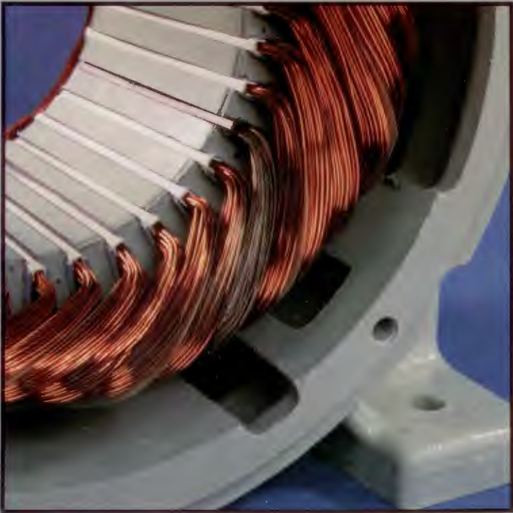
5 Winding with Shorted Coil
