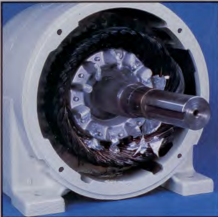
11 Damage Caused by Locked Rotor
